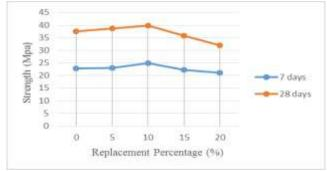
Fig 5.1: Dolomite powder compressive strength test results
