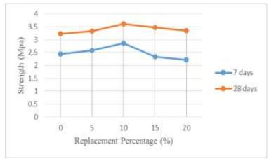
Fig 5.2: Dolomite powder split tensile strength test results
